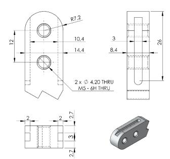
Dimensions of the gripper aluminum finger tips.
